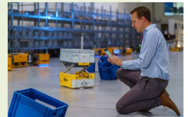
»Emili« can be controlled using a smartphone or by means of gestures: this is the prototype of the intelligent box
